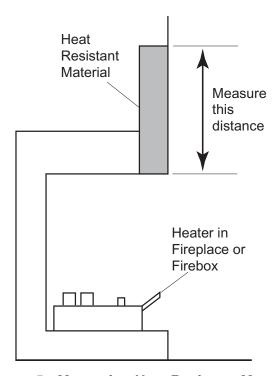
Figure 5 - Measuring Heat Resistant Material
